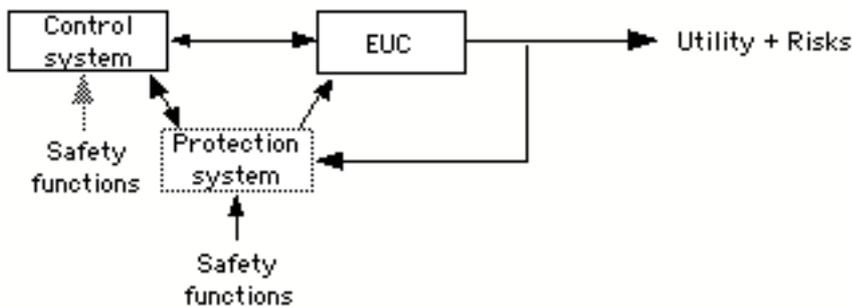
Figure 2: IEC 61508 system model
