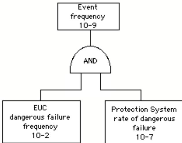
Figure 3: The principle of a protection system
